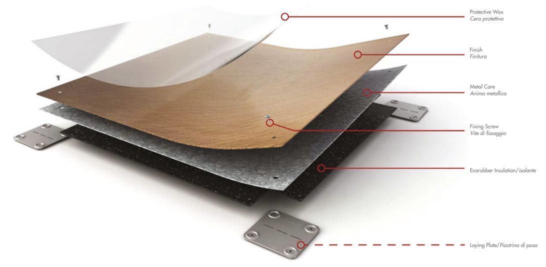
**SM02 Evolution** is a technical floor with a dry laying system. This is done by means of a support and mechanical coupling between tile and tile.
