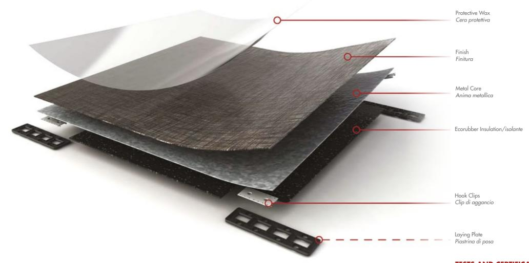
**PLO1 Invisible** is a technical floor with a dry laying system. This is done by one-click coupling between tiles. According to the criteria of the "Sustainable Project", guaranteeing well-being and attention to the environment, the one-click coupling system ensures that the installation is simple, immediate and effective, as well as reversible, if necessary.
