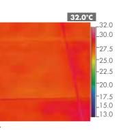
**75 min. after switching on:** I average surface module 16.8°C.
